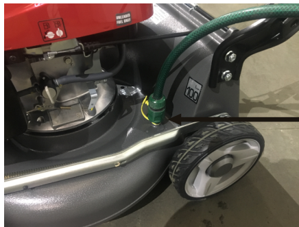
GARDEN HOSE CONNECTED TO WASH FEATURE
