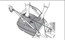
2. Put the mulch plug (A) into the discharge channel.
