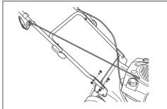
2. Lift the upper handle until it aligns with the lower handle. Tighten the knobs.
