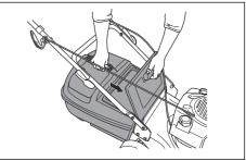
Lower the rear cover to lock the grass catcher into position.
