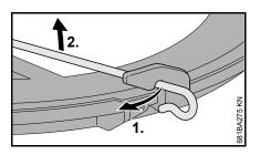
Disconnect wire rod from the transport guard.
