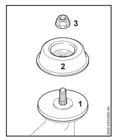
Depending on the cutting attachment, it may be necessary to use the nut (3) and rider plate (2). The thrust plate (1) must be used with all cutting attachments.
