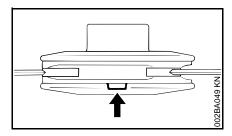
If one of the wear limit marks on the PolyCut mowing head is worn through (arrow): Do not continue using the mowing head. Install a new one. There is otherwise a **risk of injury** from thrown parts of the head.
