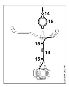
Push the throttle cable (14) into the retainers (15).
