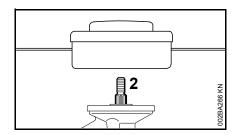
Only mowing heads may be used which mount directly to the shaft (2).
