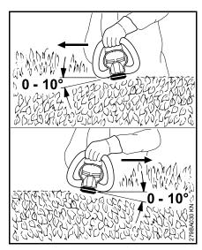
Hold the cutting blade at an angle of 0° to 10° as you swing the hedge trimmer horizontally, using both sides of the blade
