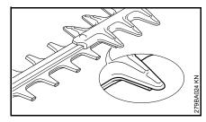
The blades are partly covered by the blade guard in the idle position.
