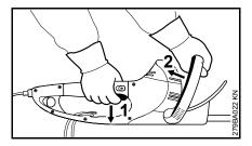
Release the trigger switch (1) and the switch lever (2).
