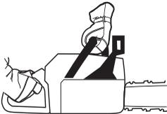
Apply full throttle and activate the chain brake by tilting your left wrist forward onto the front hand guard. Do not let go of the front handle. **The chain should stop immediately.**
