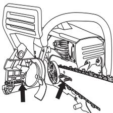
Tension the chain by turning the chain tensioning screw clockwise using the combination spanner. The chain should be tensioned until it does not sag from the underside of the bar.
