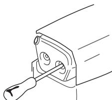
Some mufflers are equipped with a special spark arrestor mesh. If your machine has this type of muffler, you should
