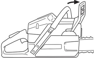
**Starting:** The chain brake must be engaged when the chain saw is started. Activate the brake by moving the front hand guard forwards.
