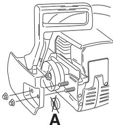
Fit the bar over the bar bolts. Place the bar in its rearmost position. Place the chain over the drive sprocket locate it in the groove on the bar. Begin on the top edge of the bar.
