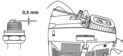
Note! Always use the recommended spark plug type! Use of the wrong spark plug can damage the piston/cylinder. Check that the spark plug is fitted with a suppressor.
