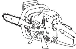
**IMPORTANT!** In order to maintain operation of the centrifugal cleaning system it must be regularly maintained. Clean the air intake to the starter, the fins on the flywheel, the space around the flywheel, inlet pipe and carburettor compartment.
