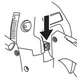
NOTE! The start/stop switch automatically returns to run position. To avoid involuntary start up, the spark plug cap must always be removed from the spark plug when the machine is unsupervised.
