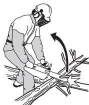
Have control over the workpiece. If the pieces you intend to cut are small and light, they can jam in the
