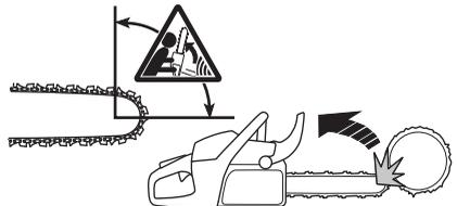
Kickback always occurs in the cutting plane of the bar. Normally the chain saw and bar are thrown backwards and upwards towards the user. However, the chain saw may move in a different direction depending on the way it was being used when the kickback zone of the bar touched the object.
