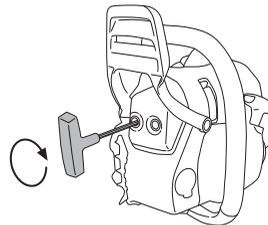
Some mufflers are equipped with a special spark arrester mesh. If your machine has this type of muffler, you should clean the mesh at least once a week. This is best done with a wire brush. A blocked mesh will cause the engine to overheat and may lead to serious damage.
