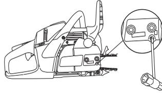
The chain is correctly tensioned when it does not sag from the underside of the bar, but can still be turned easily by hand. Hold up the bar tip and tighten the bar nuts with the combination spanner.
