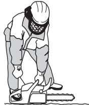
**NOTE!** Do not pull the starter cord all the way out and do not let go of the starter handle when the cord is fully extended. This can damage the machine.
