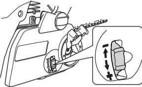
The chain is correctly tensioned when it does not sag from the underside of the bar, but can still be turned easily by hand. Hold up the bar tip and tighten the bar knob by turning the knob clockwise.
