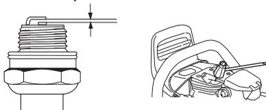
Note! Always use the recommended spark plug type! Use of the wrong spark plug can damage the piston/cylinder. Check that the spark plug is fitted with a suppressor.
