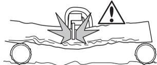
Start by cutting from above (about 1/3 of the way through). Finish by cutting from below so that the two cuts meet.
