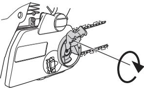
When fitting a new chain, the chain tension has to be checked frequently until the chain is run-in. Check the chain tension regularly. A correctly tensioned chain ensures good cutting performance and long life.
