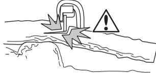
Start by cutting from below (about 1/3 of the way through). Finish by cutting from above so that the two cuts meet.
