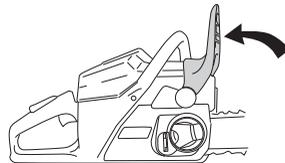
Remove the knob and remove the clutch cover (chain brake). Take off the transportation ring.
