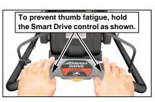
After maximum ground speed is obtained, applying additional pressure will not further increase ground speed. Apply only enough pressure to achieve the desired speed.
