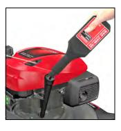
If you don't use the supplied oil, add enough SAE 10W-30 API service category SJ or later oil to bring the oil level between the upper and lower limit marks on the dipstick—without screwing the dipstick in (approximately 0.35 L is required). See page 6.
