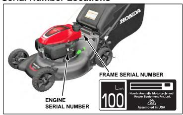
There are two serial numbers, one for the engine and one for the mower frame. Record the engine and frame serial numbers in the space below. You will need these serial numbers when ordering parts and when making technical or warranty inquiries.
