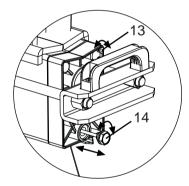
Before operating the log splitter, the Bleed Screw should be loosened by some rotations until air can go in and out of the oil tank smoothly.
