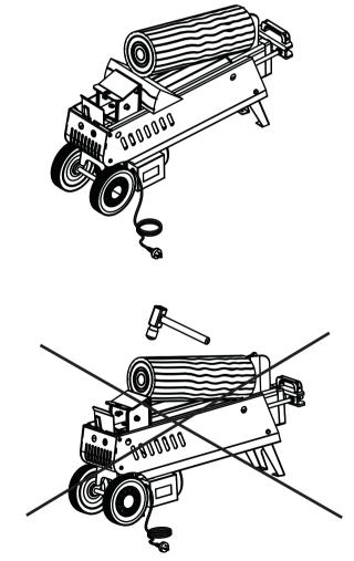
Do not try to knock the jammed log off. Knocking about will damage the machine or may launch the log and cause accident.
