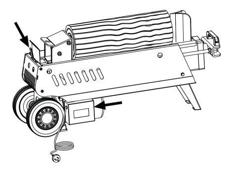
This log splitter is equipped with "ZHB" control system that requires to be operated by both hands of the user – Left hand controls the hydraulic control lever while right hand controls the pushbutton switch. The log splitter will freeze upon absence of either hand. Only after both hands release the controls, the log pusher starts to return backward to the starting position.
