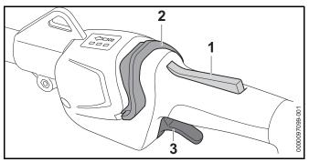
Press the trigger lockout (1) with your hand and keep it pressed.
