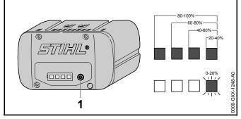
Press the button (1). The LEDs (5) glow green for about 5 seconds and indicate the state of charge.
