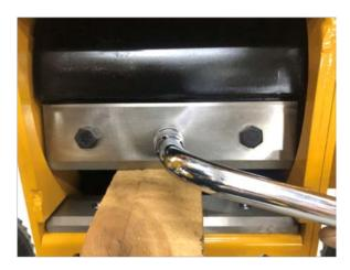
4. Remove the blade anvil (Figure 15). Give a really good clean of chipper blades and anvil and make sure there is no dirt.
