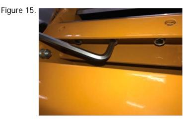
Put the anvil back to the chipper and screw on (make sure to keep anvil bolts loose as you need to adjust it later).
