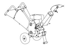
Step 5. – Connect the emergency cable. Fix the switch box by tightening the two bolts (A), and then connect the cable plug.
