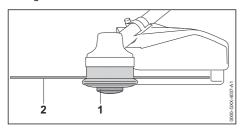
Automatic feed will not take place if the mowing lines are shorter than 25 mm.
