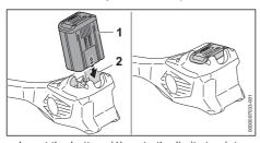
Insert the battery (1) up to the limit stop into the battery compartment (2).
